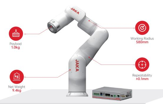
The JAKA Minicobo is compatible with Ethernet protocols (TCP/IP) and control interfaces such as Modbus and Profinet. It can simply and quickly integrate end effectors, grippers, suction, vision systems and force control modules. JAKA also provides an ROS package and SDK secondary development package, meaning that operators can quickly adapt the cobot to suit new or experimental applications.
